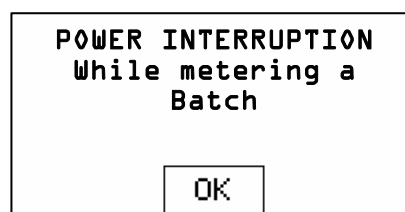
Figure 44: Typical "Power Interruption" Alarm Screen
